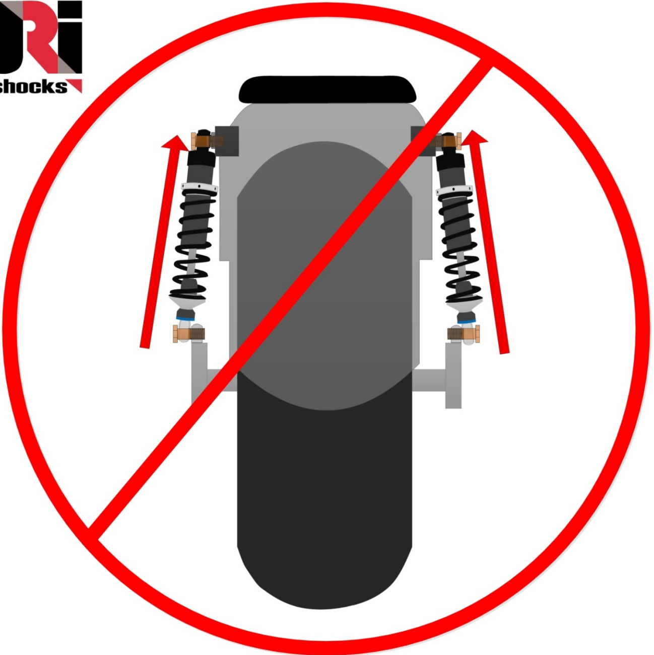
Figure 7 - DON'T INSTALL SHOCKS AT AN ANGLE
