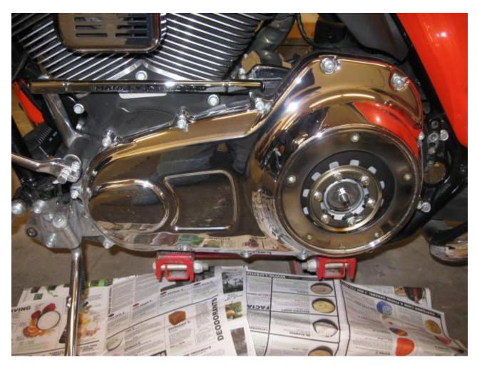
Remove the outer primary cover. Zip tie the chain tensioner and remove the two mounting bolts...be aware that there are two "spacers" that go between the tensioner and the case...they may remain on the tensioner (one of mine fell off, while the other remained attached) they're on the backside of the tensioner where the bolts go through. If they don't stay on the tensioner make sure you keep tabs on them and they are in place once you reinstall the tensioner.
