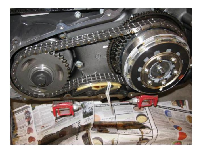
You need to make a sprocket locking tool, I used a 1X2 piece of wood cut to  $6\ 1/4$ " length which worked nicely. Put it between the comp sprocket and clutch assembly like shown in the pic below.
