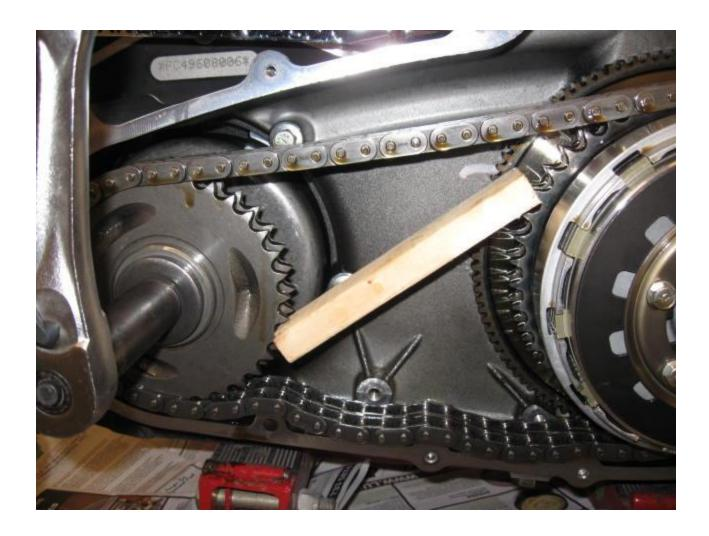
You need a 13/16" socket to remove the stock comp bolt. It's on there pretty good and I ended up using a breaker bar to crack it loose. Once the bolt is out simply remove the stock shaft extension, this will free up the stock comp sprocket and allow you to remove the chain without having to remove the clutch assembly. Use care to not bind up the chain. There's plenty of slack and room to store the chain safely off to the clutch side of the primary.
