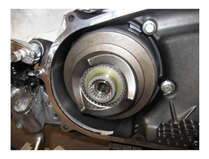
Followed by the SE comp sprocket. Obviously you'll have to slip the chain back on before sliding the sprocket onto the smooth bearing journal of the shaft extension.
