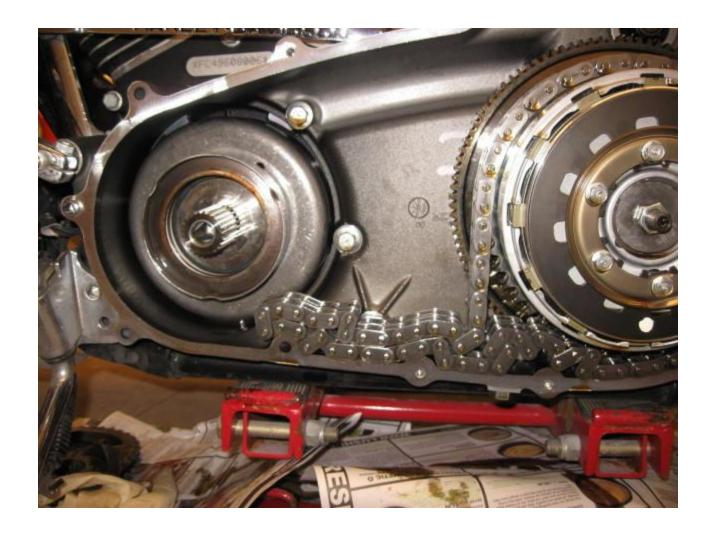
Here comes the part when you have to remove/grind material from the primary case to allow the rotor to be removed. I used a die-grinder with a cone shaped de-burring bit. Not much material needs to be removed and the total time to grind was less than 3 minutes. The pic below shows why grinding is needed.
