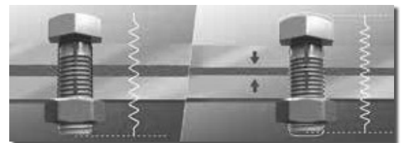
Stretching of the bolt beyond its yield point and thermal expansion/contraction of parts lead to lack of structural rigidity and relaxation of parts.
