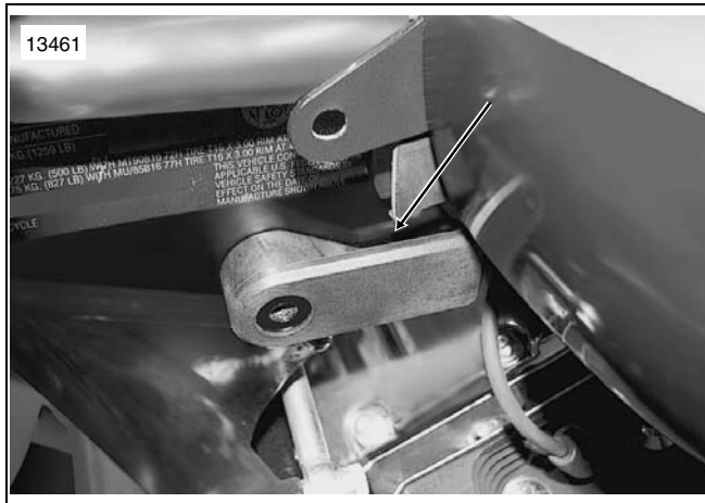
Figure 4. Left Hand Fuel Tank Brace with Cutout
