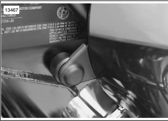
Figure 8. Front Fuel Tank Fastener Boot Installed
