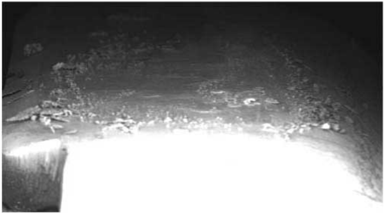
Figure 3. View of Fretting on Pins
