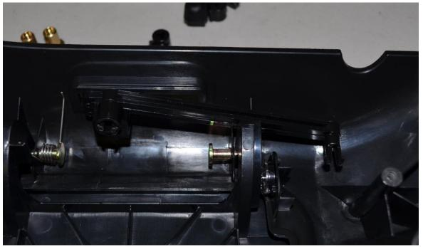
Step 18: Install inner glove box (F1 or F2) onto the glove box surround (B1 or B2) using three Phillips head self tapping screws (16)
