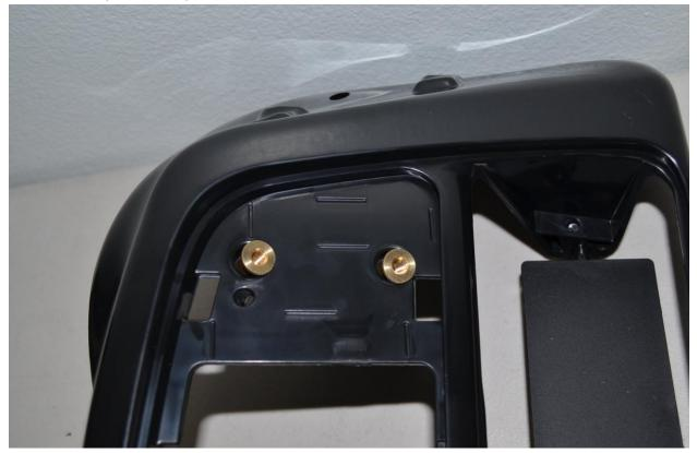
Step 5: While holding the brass insert (25) with one hand, thread in the large Allen head screws (13). Tighten the screw to pull the brass insert into the outer fairing (A1 or A2) until the insert is about 1MM below flush with the surface. Use a large washer (17) to prevent damage to the plastic. DO NOT OVERTIGHTEN THESE, YOU CAN CRACK THE PLASTIC.
