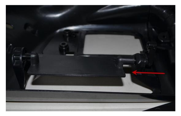
Step 4: Insert the brass inserts (25) into the outer fairing (A1 or A2). These will not fit snugly in the holes, and cannot be pressed in by hand.
