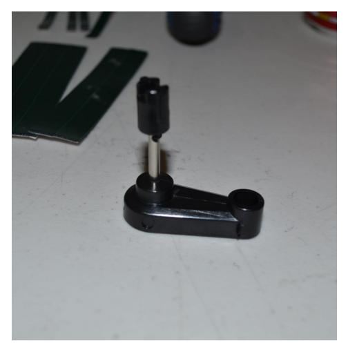
Step 2: Insert plastic vent door hinge pins (8) into the flat vent door tab on left or right outer fairing (A1 or A2)
