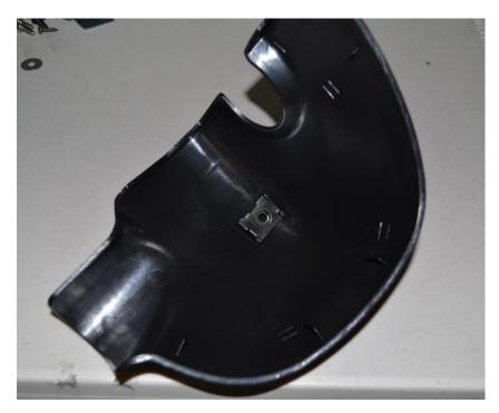
Working through the open glove box, install the 10MM bolts (12) into the speed nuts (11) to attach your fairing caps.
