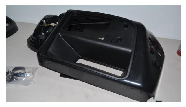
Step 9: Install the front bezel cover (H1 or H2) onto the fairing assembly (A1 or A2 and D1 or D2) by inserting the three tabs on the bottom into the three slots in the front bezel and push in the top tabs until they lock into place.
