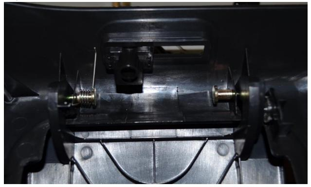
Step 16: Assemble vent lever sliders and vent lever knobs (19 and 20) onto the glove box surrounds (B1 or B2) using the T25 Torx head screws (7)
