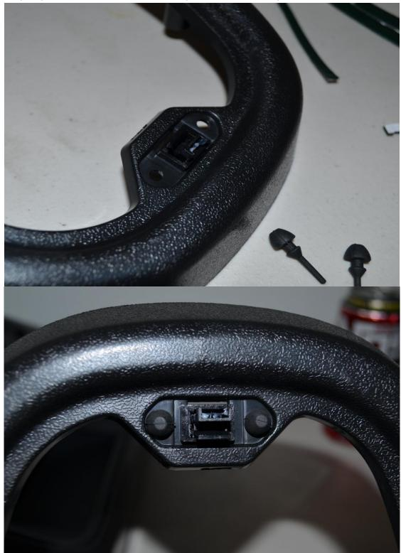
Step 11: Push in the glove box door clips (14) into the glove box surrounds (B1 or B2) and pull the rubber bump stops (5) into the holes next to the clips. Ensure that the clip is in the correct orientation.
