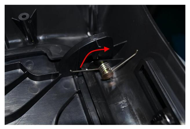
Step 15: Install other glove box pin (24) into other side, through the tab on the glove box surround and the glove box door (B1 and B2 or E1 and E2)
