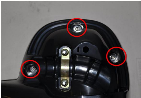
This concludes the assembly off the bike for your lower vented fairings. To mount these to your bike, remove the two 10MM nuts and mounting bracket (26), install the lower vented fairing, then replace the mounting bracket and two 10MM nuts (26) and tighten them down.
