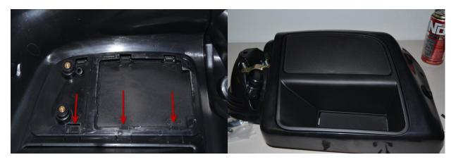
Step 10: Install inside panel (C1 or C2) to the corresponding fairing assembly, using the large Allen head screws (13) and large washers (17) into the brass inserts (25).
