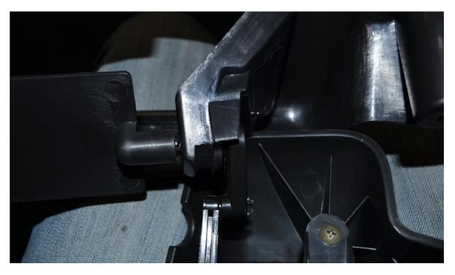
Step 19: Clip vent linkage (23) into the assembled vent door arm and actuator rod (18 and 21)
