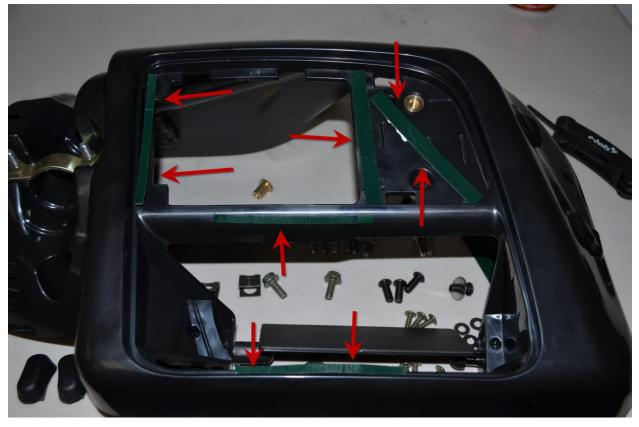
Step 8: Install the front bezel (D1 or D2) to the corresponding outer fairing (A1 or A2). Once the piece is installed, you will not be able to remove this piece.
