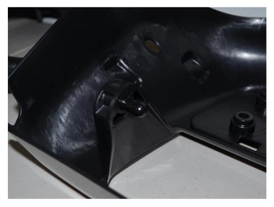
Step 3: Install the vent door onto the plastic vent door hinge (8), and insert the assembled vent door arm and actuator rod (18 and 21) into the assembly through the offset vent door tab
