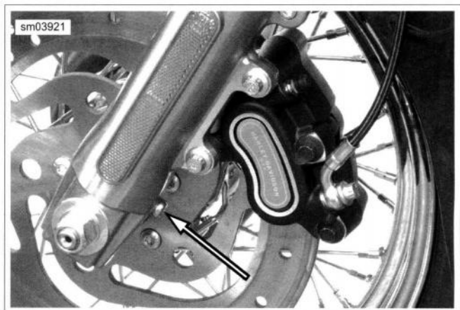
Figure 2-68. Fork Drain Screw: (Left Side Shown)
