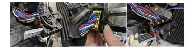
J. Push Grey pin lock back into lock position. Ziptie or route in OEM wire cover to keep wire safe from damage.
