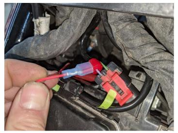
G. Connect BAS Black wire to ground stud front left of the battery.
