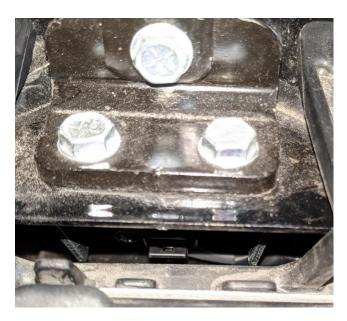
E. Connect the BAS bracket assembly to above screws pictured above^
